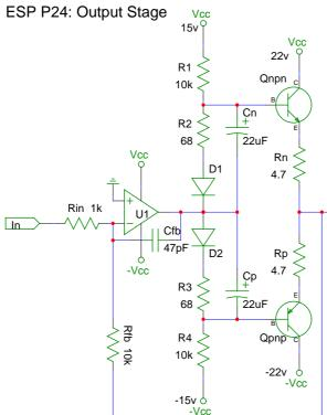
Qnpn+Qpnp are Class AB, 80mA, and will need a heat sink. The entire booster is in the op amp feedback loop. This allows for better tracking by the op amp (less distortion).
