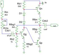
Transistor Radio Amp (Class B Inverted, 50mW estimated, 30mA from 9v battery)
