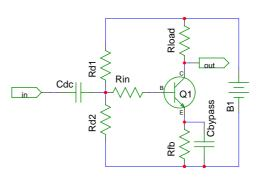
Standard Class A Amp with AC Bypass This amp has a feedback resistor for DC to prevent thermal runaway. It is bypassed with Obypass thus allowing AC signals to pass unimpeded. DC signals are forced through Rfb since the capacitor won't allow them to pass. AC signals are amplified at whatever the beta is for the transistor. Rfb lowers the DC gain to something very small to help prevent heat build up.
