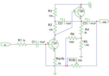
Modified ESP13 Mic PreAmp (600 ohm, Class A, inverted output)
