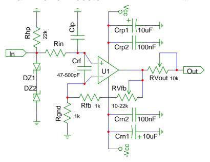
This is a simple amplifier capable of handling frequencies down to DC.
