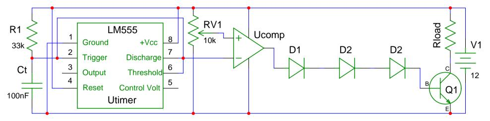
The LM555 produces a sawtooth waveform that gets sent to the op-amp.
