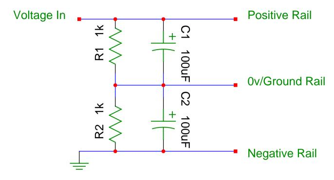
This is a quick and simple way of getting a dual rail voltage supply.
