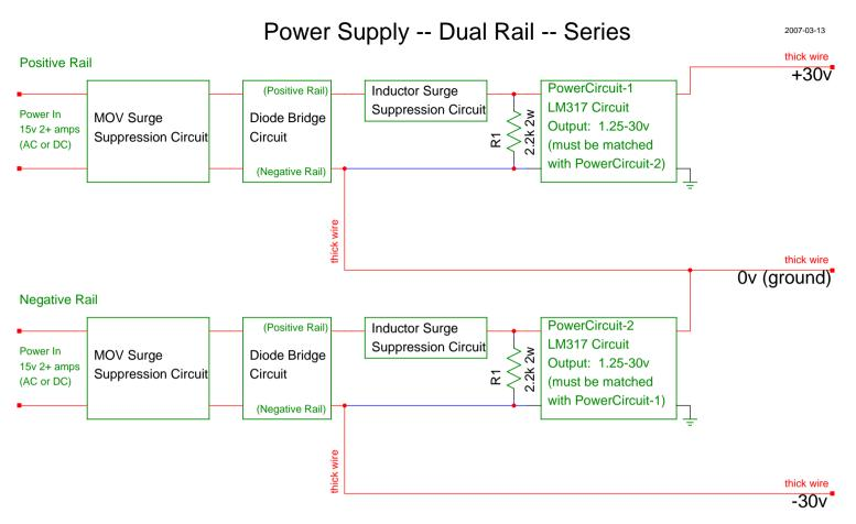
"Power In" MUST be independent secondaries from a transformer or 2 different wall warts/floor frogs.
