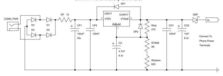
This is a simple 3x AA battery eliminator circuit for use with cordless telephones (but can be used with other low current devices). If parts are tightly packed together, the main circuit board will be about 1.5"x0.5".
