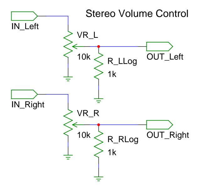
If real log pots cannot be found, use R\_xLog resistors to simulate it. R\_xLog should be 1/6 to 1/10 the value of VR\_x and VR\_x is 10x greater than the source impedance. Using the shunt resistor will present varying impedance to the amp.
